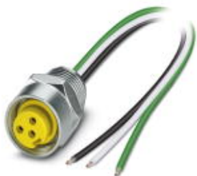
Flush-type connector, 3-position, Socket, straight, 7/8"-16UNF, on free cable end, Front mounting, with 1/2 inch-14 NPT mounting thread, Individual wires, cable length: 1 m
