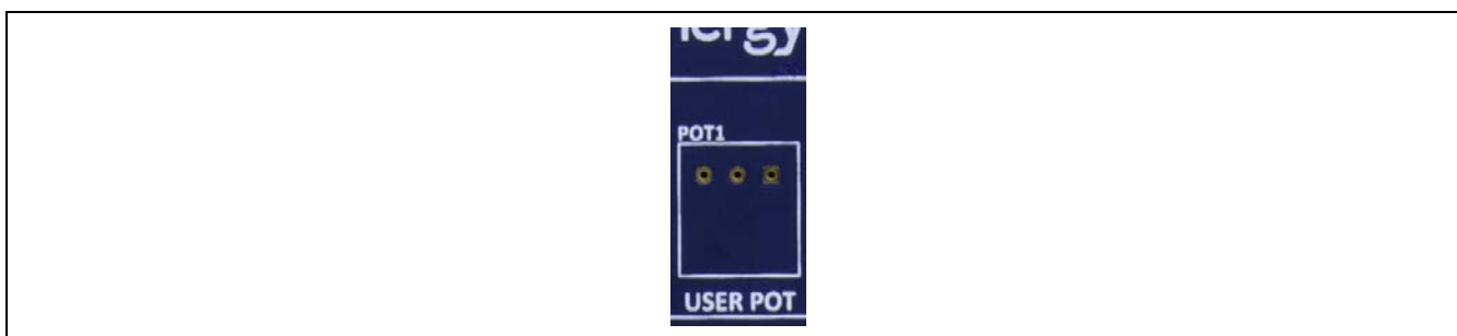
Figure 25 User potentiometer on target board (top)
