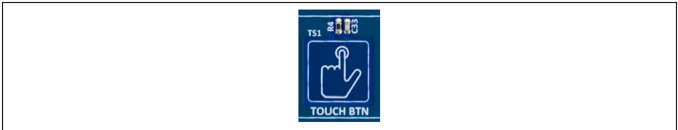
Figure 19 Capacitive touch button on target board (top)
