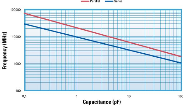
**First Resonance Frequency vs Capacitance**
