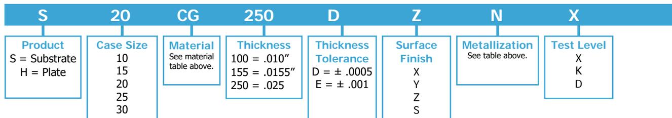
**Thickness Code.** A three digit code representing the thickness in mils.
