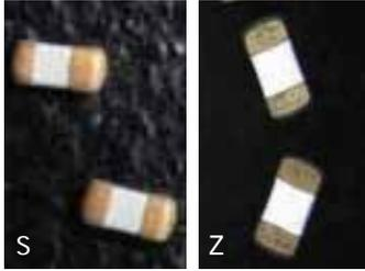
0402 product line extension of Z type plating (Sn over Ni) in the C04 (0402) case size with its Ultra-Low ESR UL dielectric material. Previously the C04 product line was only available in "S" type plating (Au flash over Ni).
