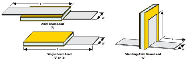
**Notes:** • See Di-Cap® Termination Code Table for available lead configurations. • Lead material is 0.002" pure silver, (Ag), 0.002" ±.0005" thick. • Leads are attached with AuSn, 80%/20% eutectic alloy. Re-flow temperature is 280°C minimum. • Pure Gold, (Au) leads are available. Consult factory for details. • Chip dimensions per Di-Cap® dimensions table. • Custom lead dimensions are available. Consult factory for details.
