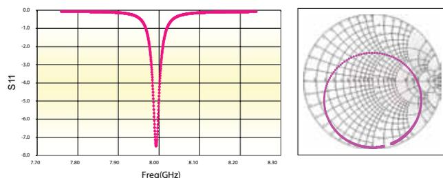
DLI resonators are direct in frequency. So in addition to all of the other benefits no multiplication is required as there would be in other technologies. As a solid block of ceramic they are also non microphonic
