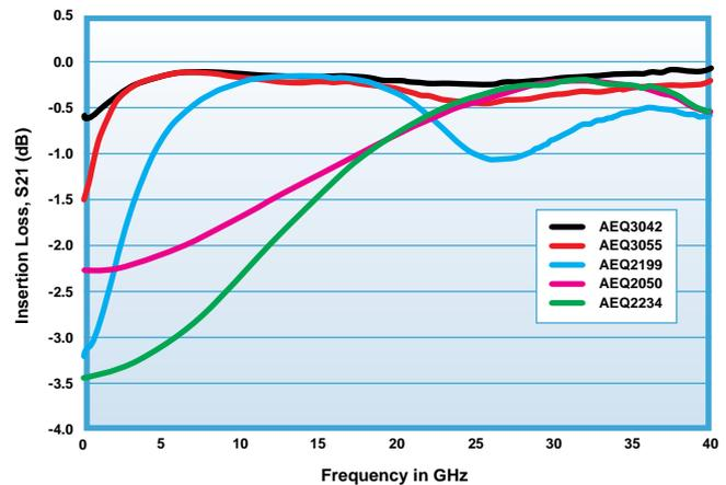
Excellent, repeatable microwave performance is achieved by application of precision thin film fabrication and DLI Hi-K Ceramic materials. DLI's unique design solution provides near Ideal R-C frequency response, far superior to "Stacked R-C chip" Assemblies.
