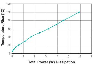
Total Power Dissipation = Copper Loss (W) + Core Loss (W)
