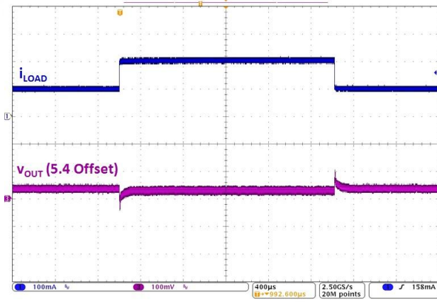
Figure 15. Load Transient, 3.6 V_{IN} , 100 \leftrightarrow 200 mA, 1 \mu\text{s} Edge
