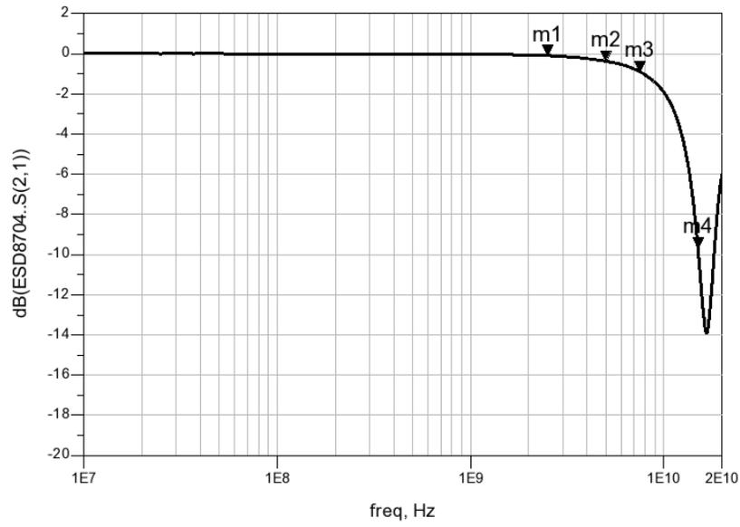
Figure 13. ESD8704 Insertion Loss
