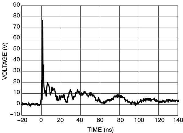
**Figure 1. IEC61000-4-2 +8 kV Contact ESD Clamping Voltage**
