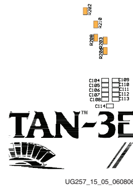
Figure 15-5: Location of Termination Resistor Pads on Bottom Side of Board
