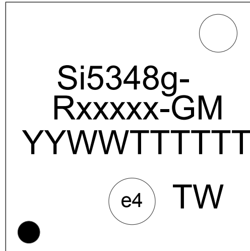
Figure 12.1. Si5348 Top Marking
