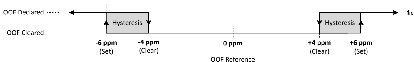
Figure 3.13. Example of Precise OOF Monitor Assertion and De-assertion Triggers
