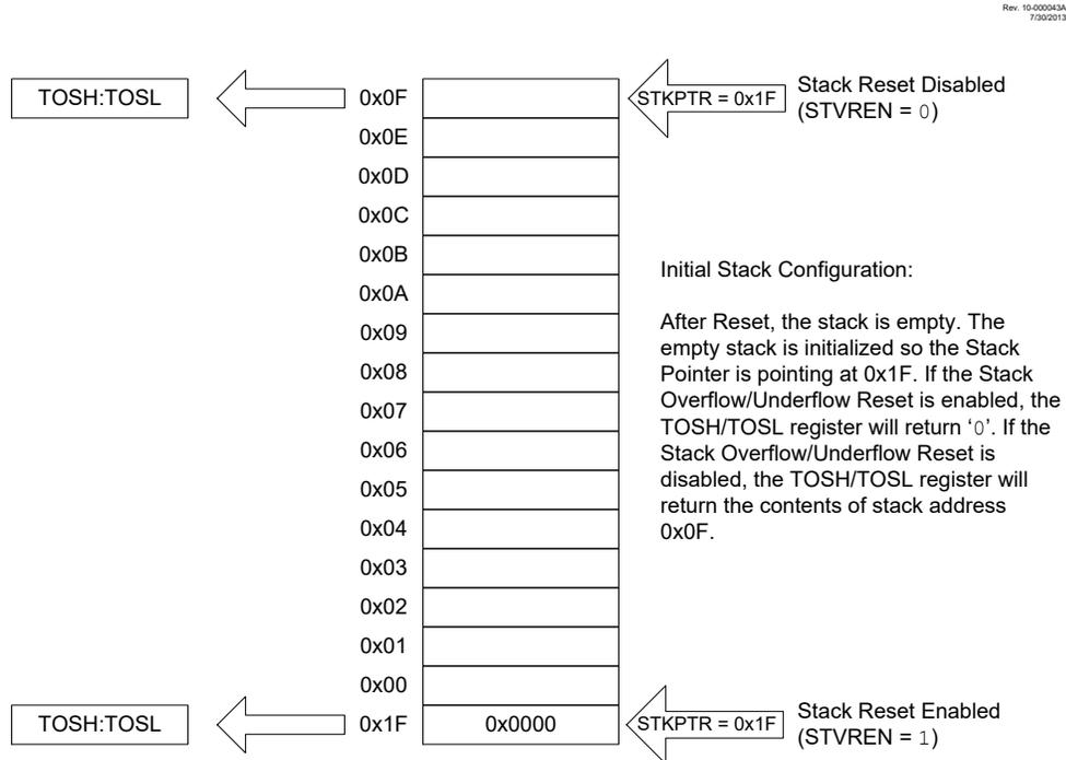
Figure 7-5. Accessing the Stack Example 2
