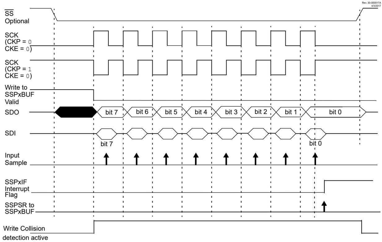
**Figure 35-8. SPI Mode Waveform (Slave Mode with CKE = 1)**
