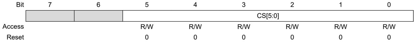
**Bits 5:0 – CS[5:0]** ADC Conversion Clock Select bits
