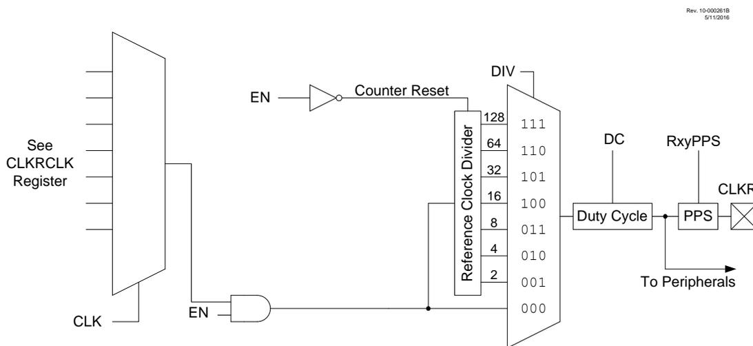
Figure 34-2. Clock Reference Timing
