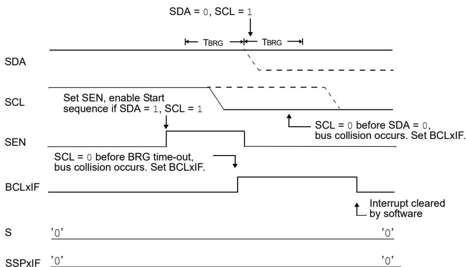
If the SDA pin is sampled low during this count, the BRG is reset and the SDA line is asserted early (Figure 35-35). If, however, a '1' is sampled on the SDA pin, the SDA pin is asserted low at the end of the BRG count. The Baud Rate Generator is then reloaded and counts down to zero; if the SCL pin is sampled as '0' during this time, a bus collision does not occur. At the end of the BRG count, the SCL pin is asserted low.
