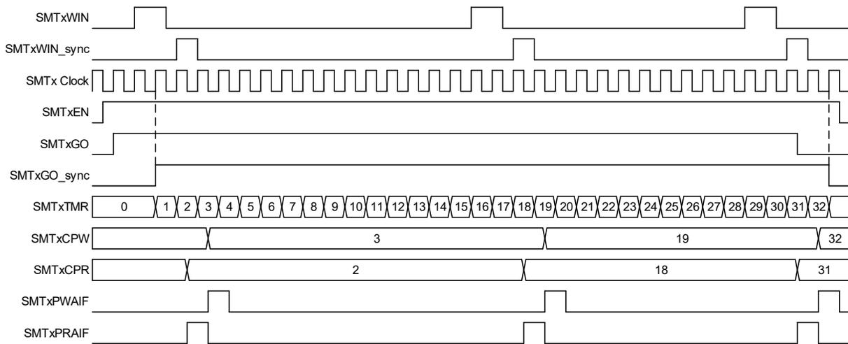
**Figure 37-16. Capture Mode, Single Acquisition Timing Diagram**
