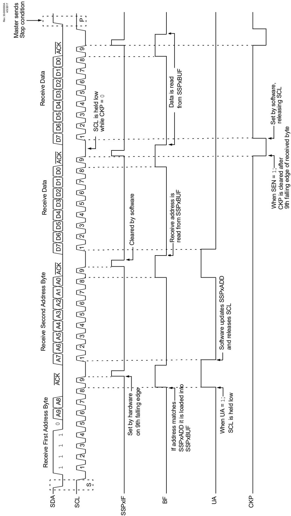
Figure 35-21. I<sup>2</sup>C Slave, 10-bit Address, Reception (SEN = 0, AHEN = 1, DHEN = 0)
