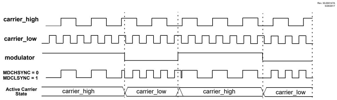
**Figure 32-6. Full Synchronization (MDCHSYNC = 1, MDCLSYNC = 1)**
