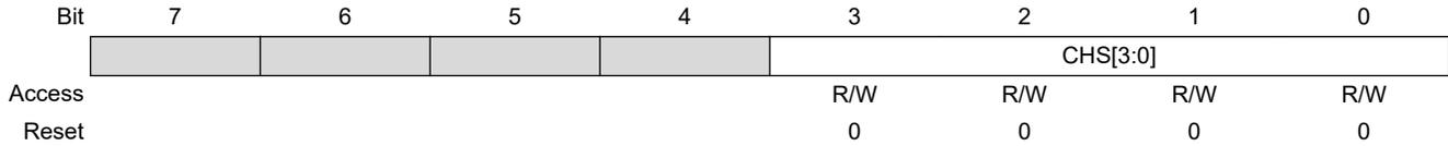
**Bits 3:0 – CHS[3:0]** Modulator Carrier High Selection bits
