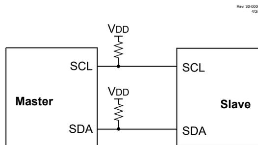
The I<sup>2</sup>C bus can operate with one or more master devices and one or more slave devices.
