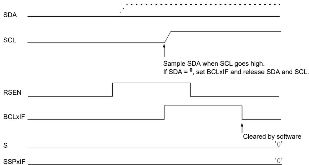
If SCL goes from high-to-low before the BRG times out and SDA has not already been asserted, a bus collision occurs. In this case, another master is attempting to transmit a data '1' during the Repeated Start condition, see [Figure 35-37](#).
