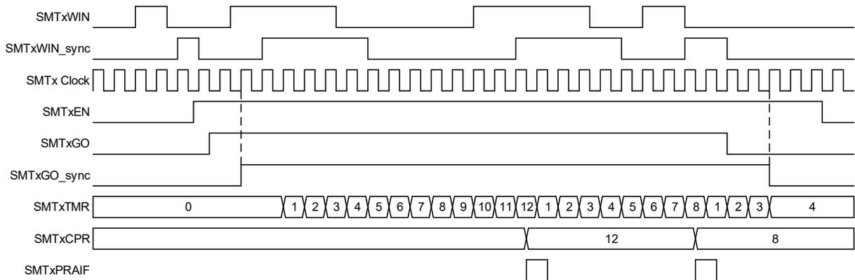
**Figure 37-10. Windowed Measurement Mode, Single Acquisition Timing Diagram**
