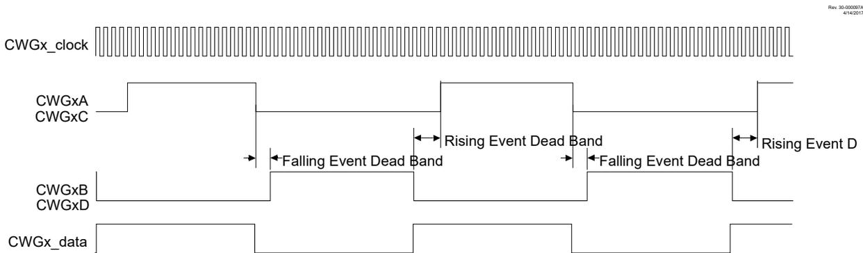
**Note:** CWGx\_rising\_src = CCP1\_out, CWGx\_falling\_src = ~CCP1\_out
