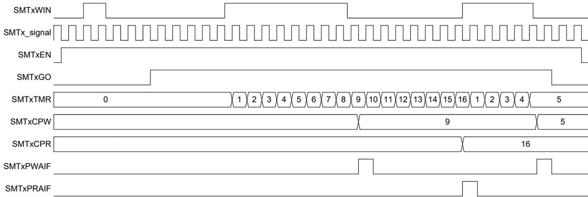
**Figure 37-21. Windowed Counter Mode, Single Acquisition Timing Diagram**
