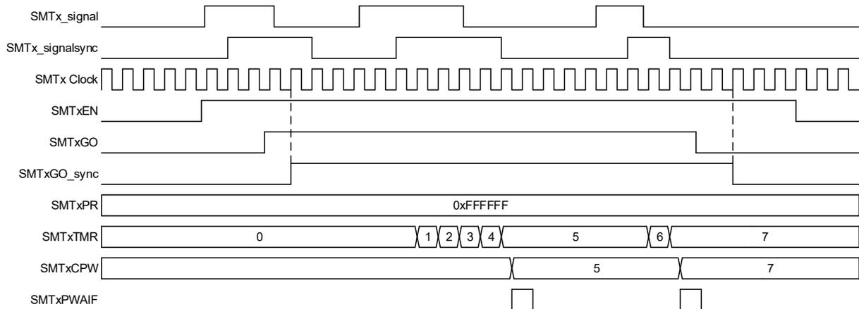
**Figure 37-4. Gated Timer Mode, Single Acquisition Timing Diagram**
