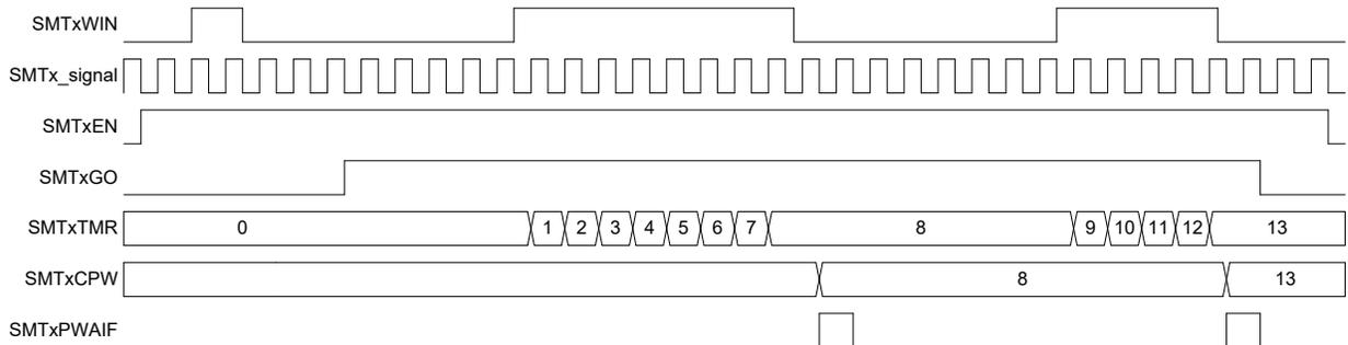
**Figure 37-19. Gated Counter Mode, Single Acquisition Timing Diagram**
