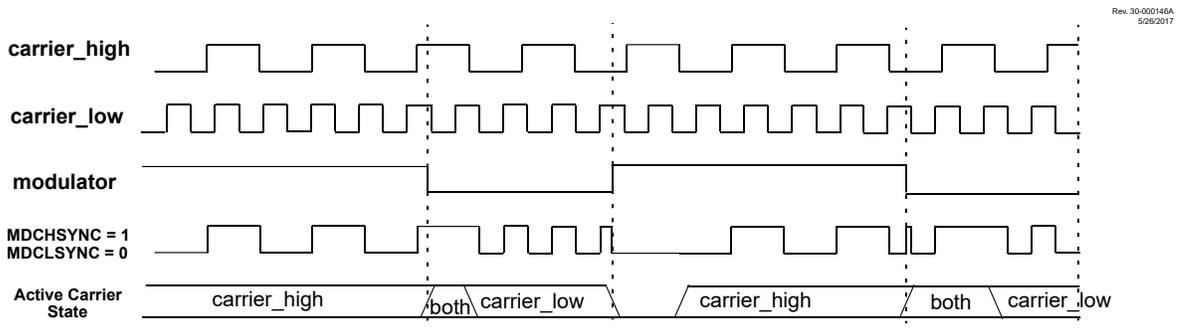
**Figure 32-5. Carrier Low Synchronization (MDCHSYNC = 0, MDCLSYNC = 1)**
