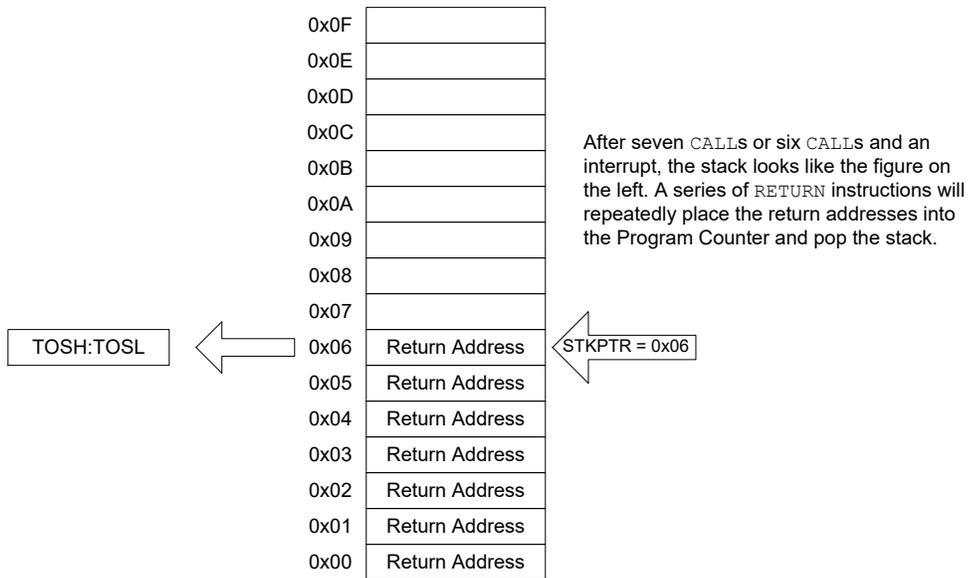
Figure 7-7. Accessing the Stack Example 4
