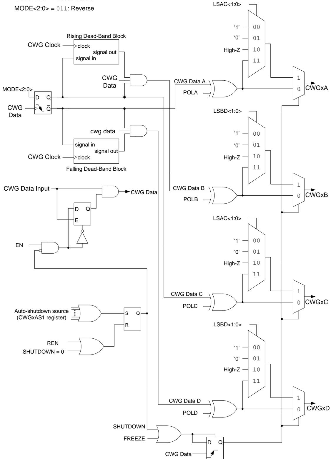
In Forward Full-Bridge mode ( $MODE = 010$ ), CWGxA is driven to its active state, CWGxB and CWGxC are driven to their inactive state, and CWGxD is modulated by the input signal, as shown in Figure 31-7.
