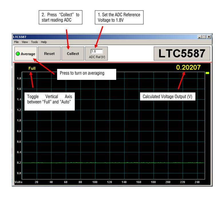
Figure 3. Front Control Panel for LTC5587. With no RF input signal.
