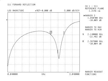
Figure 1. Standard Demo Board Return Loss
