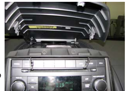
Cover Removal and screws under cover
