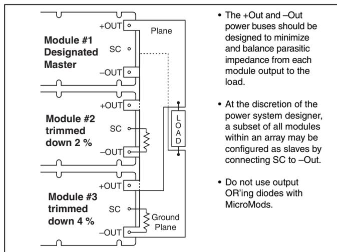
Figure 11 — N+1 module array output connections.
