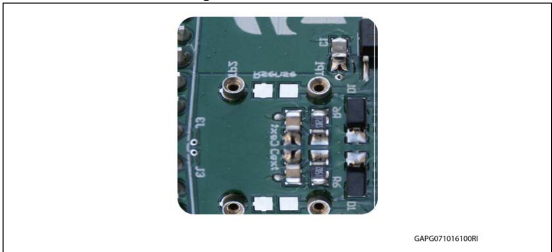
Figure 4. Mounting through-hole sense resistor
