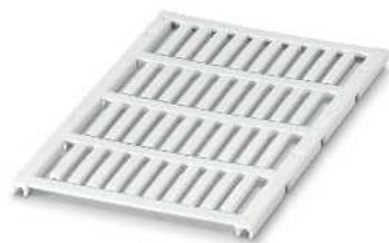
40 markers for conductor diameters from 1.3 to 1.6 mm, lettering field size: 21 x 3 mm
