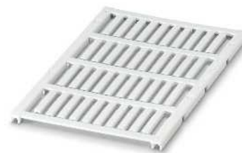
40 markers for conductor diameters from 1.6 to 2.1 mm, lettering field size: 21 x 3 mm
