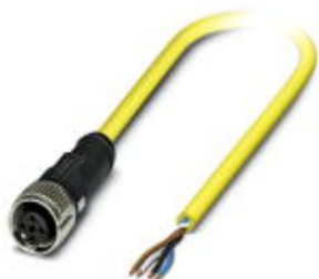
Sensor/actuator cable, 4-position, PVC, yellow, free cable end, on Socket straight M12 SPEEDCON, A-coded, cable length: 2 m
