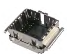
SMIA85, 7.50 by 7.50mm, 18 circuits Through-board, 5.25mm height (Series 78725)
