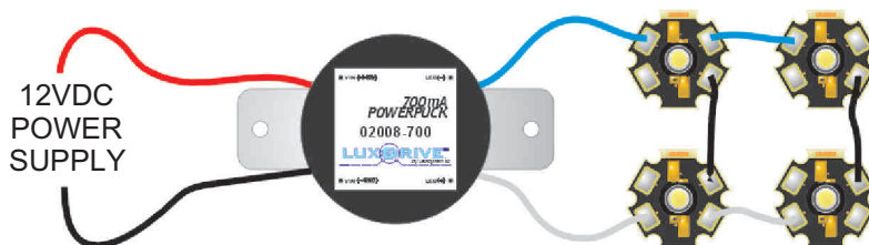
PowerPuck 2008-700 driving (4) Luxeon I LEDs from 12VDC.
