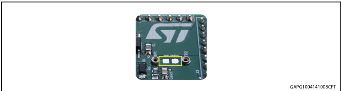
Figure 5: Pads for soldering SMD resistor
