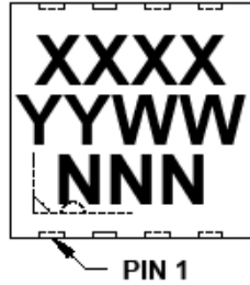
8-Lead DFN (3x3x0.9 mm)
