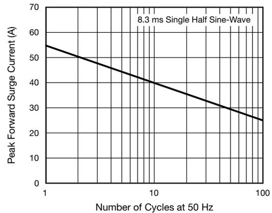
Fig. 3 - Max. Non-Repetitive Peak Forward Surge Current
