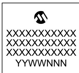
44-Lead QFN (8x8x0.9 mm)
