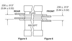
5/6. With plug assembly front mounted and receptacle assembly rear mounted, use hardware from Figures 5 and 6. If float mounting is desired, use Figure 3 or 4 for the float mounted connector.
