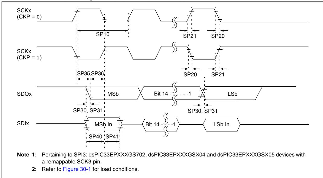
**TABLE 30-34: SPI1, SPI2 AND SPI3 MASTER MODE (FULL-DUPLEX, CKE = 0, CKP = x, SMP = 1) TIMING REQUIREMENTS<sup>(5)</sup>**
