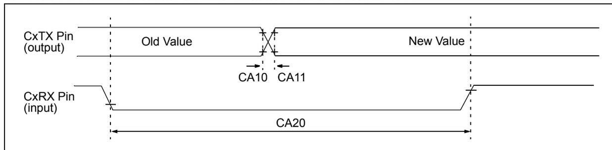
**TABLE 30-49: CANx MODULE I/O TIMING REQUIREMENTS**
