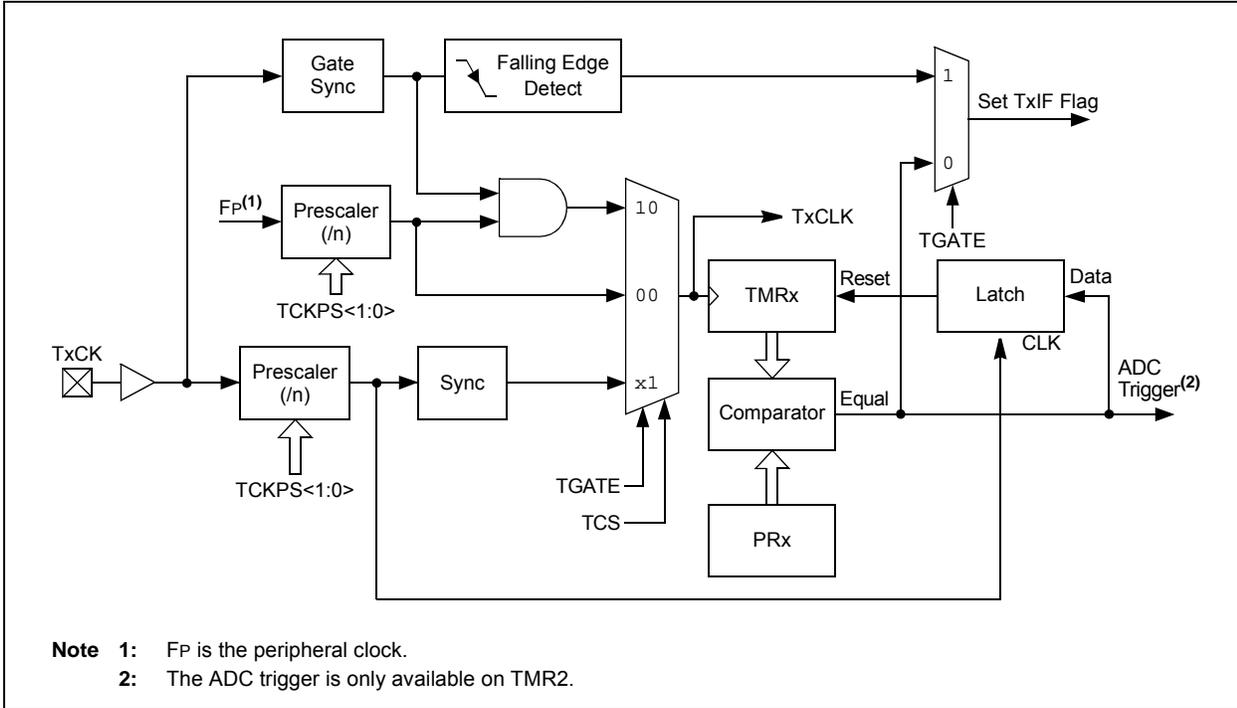
**FIGURE 13-2: TYPE B/TIME C TIMER PAIR BLOCK DIAGRAM (32-BIT TIMER)**
