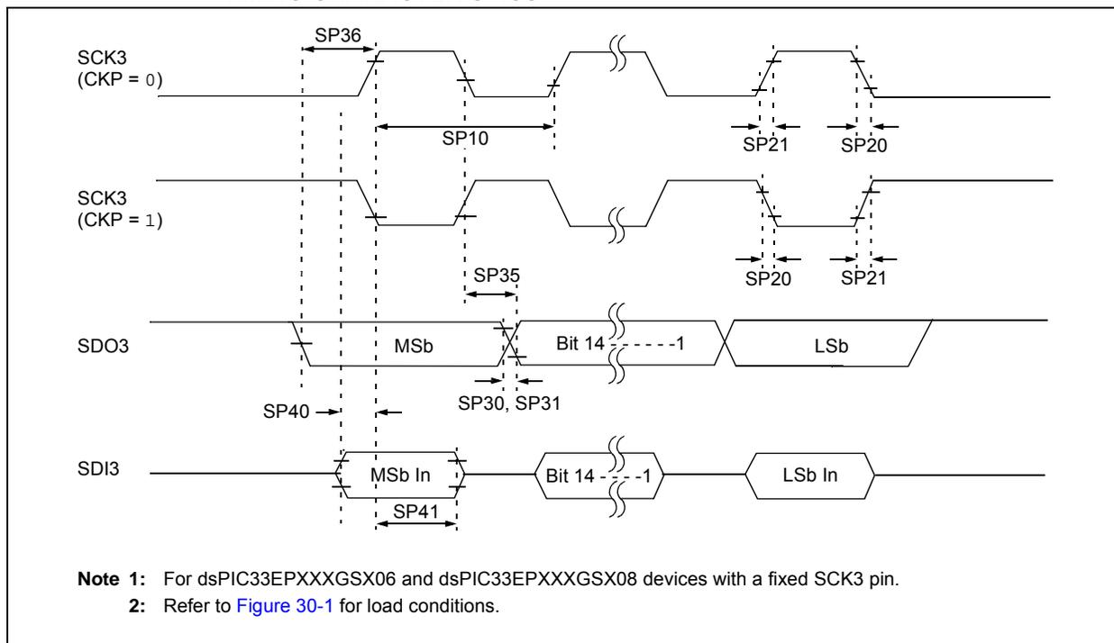
**TABLE 30-41: SPI3 MASTER MODE (FULL-DUPLEX, CKE = 1, CKP = x, SMP = 1) TIMING REQUIREMENTS<sup>(5)</sup>**
