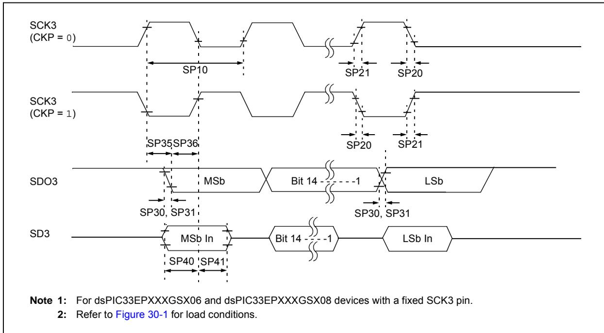
**TABLE 30-42: SPI3 MASTER MODE (FULL-DUPLEX, CKE = 0, CKP = x, SMP = 1) TIMING REQUIREMENTS<sup>(5)</sup>**
