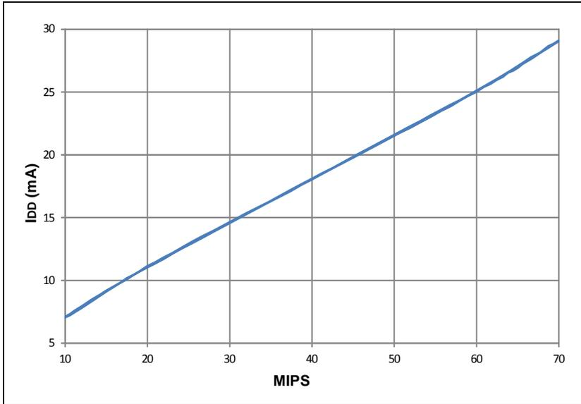
**FIGURE 31-8: TYPICAL I<sub>IDLE</sub> CURRENT @ V<sub>DD</sub> = 3.3V, +25°C**
