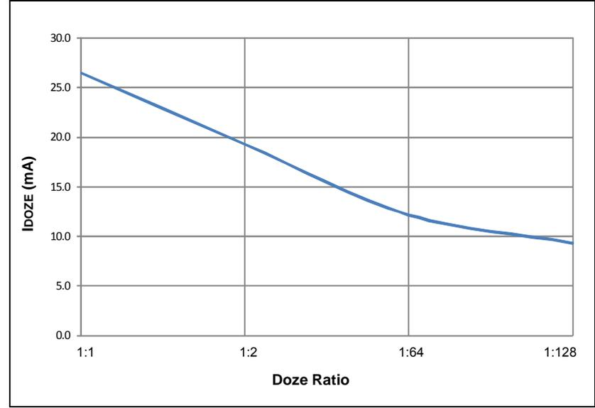
**FIGURE 31-6: TYPICAL I<sub>DD</sub> CURRENT @ V<sub>DD</sub> = 3.3V, +25°C**
