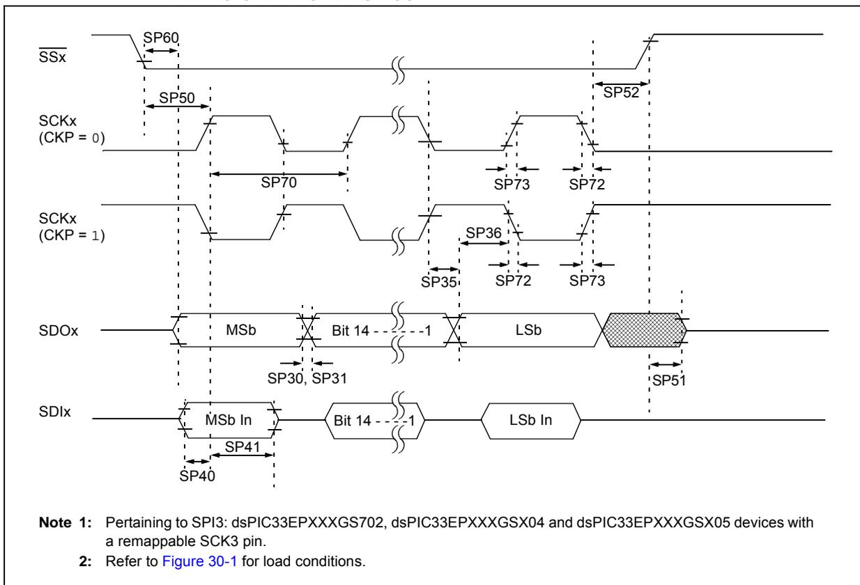
**Note 1:** Pertaining to SPI3: dsPIC33EPXXXGS702, dsPIC33EPXXXGSX04 and dsPIC33EPXXXGSX05 devices with a remappable SCK3 pin.
