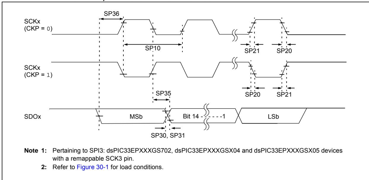
**TABLE 30-32: SPI1, SPI2 AND SPI3 MASTER MODE (HALF-DUPLEX, TRANSMIT ONLY) TIMING REQUIREMENTS<sup>(5)</sup>**
