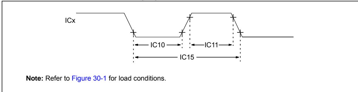
**TABLE 30-27: INPUT CAPTURE x MODULE TIMING REQUIREMENTS**
