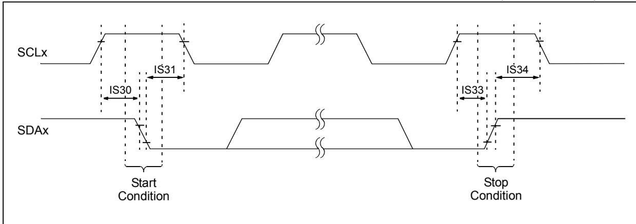
**FIGURE 30-30: I2Cx BUS DATA TIMING CHARACTERISTICS (SLAVE MODE)**
