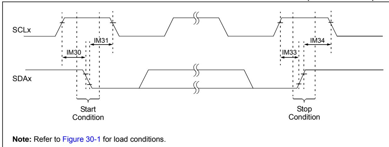
**FIGURE 30-28: I2Cx BUS DATA TIMING CHARACTERISTICS (MASTER MODE)**
