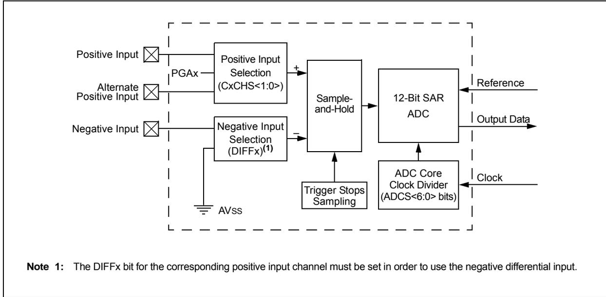
**FIGURE 22-3: SHARED ADC CORE BLOCK DIAGRAM**
