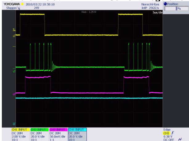
Ch 1 (yellow) – PWM signal at 30 kHz 25% duty cycle Ch 2 (green) – SW node voltage, Ch 3 (red) – LED Current. Ch 4 (blue) - V_{OUT}
