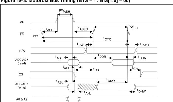
Figure 19-3. Motorola Bus Timing (BTS = 1 / BIS[1:0] = 00)
