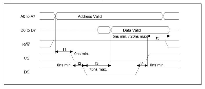
Figure 19-7. Motorola Bus Write Timing (BTS = 1 / BIS[1:0] = 01)
