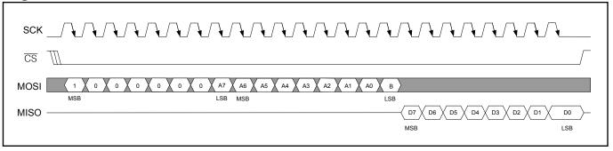
Figure 17-4. SPI Serial Port Access, Read Mode, CPOL = 1, CPHA = 1
