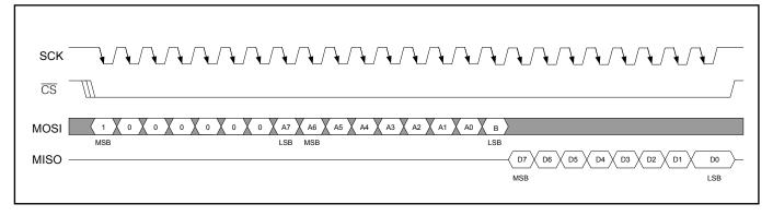
Figure 17-3. SPI Serial Port Access, Read Mode, CPOL = 0, CPHA = 1
