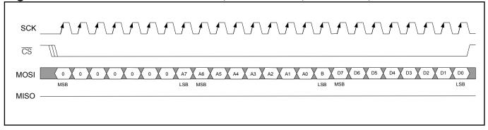
Figure 17-6. SPI Serial Port Access, Write Mode, CPOL = 1, CPHA = 0
