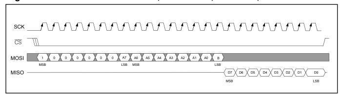
Figure 17-2. SPI Serial Port Access, Read Mode, CPOL = 1, CPHA = 0
