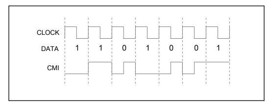
Transmit and receive CMI is enabled via LIC4.7. When this register bit is set, the TTIP pin will output CMI-coded data at normal levels. This signal can be used to directly drive an optical interface. When CMI is enabled, the user can also use HDB3/B8ZS coding. When this register bit is set, the RTIP pin will become a unipolar CMI input. The CMI signal will be processed to extract and align the clock with data.
