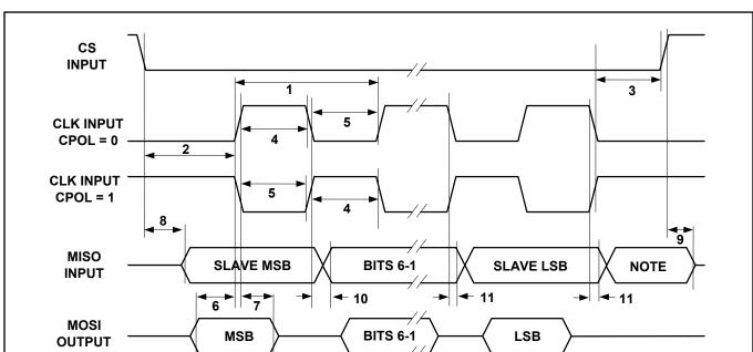
Figure 19-8. SPI Interface Timing Diagram, CPHA = 0, BIS[1:0] = 10
