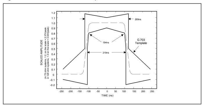
Figure 13-7. T1 Transmit Pulse Template
