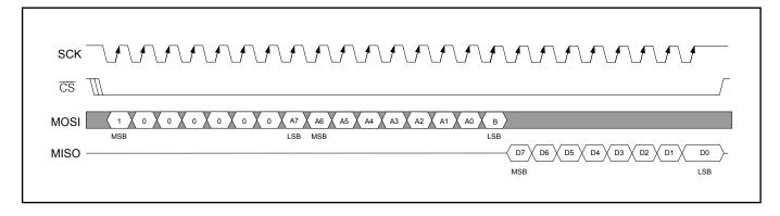
Figure 17-5. SPI Serial Port Access, Write Mode, CPOL = 0, CPHA = 0
