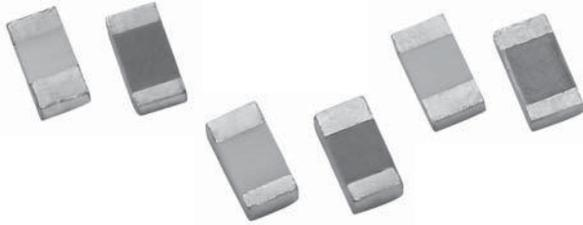
Thin Film Mil chip resistors feature all sputtered wraparound termination for excellent adhesion and dimensional uniformity. They are ideal in applications requiring stringent performance requirements. Established reliability is assured through 100 % screening and extensive environmental lot testing.
