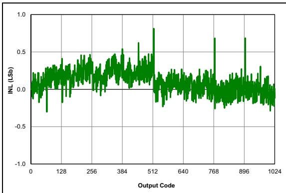
FIGURE 36-68: ADC 10-bit Mode, Single-Ended INL, V_{DD} = 3.0V , T_{AD} = 4\ \mu\text{s} , 25^\circ\text{C} .
