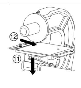
Tighten screws securely, in order (after table is placed back onto press).
