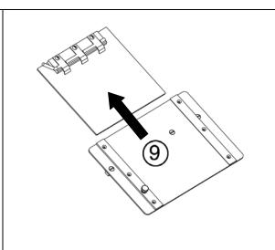
\* Select the mating rack for the installed character dial. <u>Slightly</u> tighten screws.
