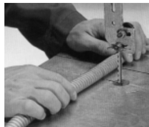
Position conduit at right-angle to band saw
