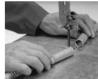
Conduit ends are clean and ready for use
