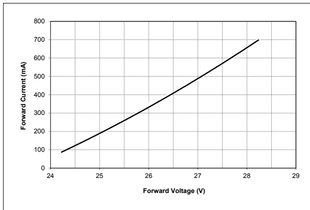
Figure 3: Vero SE 10D Drive Current vs. Voltage
