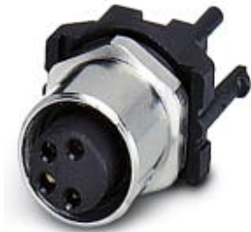
Sensor/actuator flush-type socket, 4-pos., M8, rear/screw mounting with M8 thread, polarity protection, with straight solder connection, model with 6 mm long terminal pins
