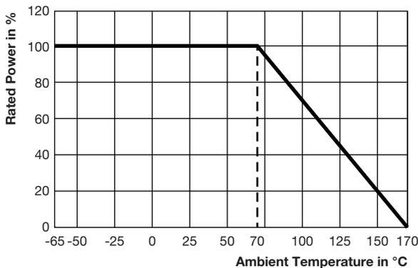
Fig. 1 - Ambient Temperature Derating
