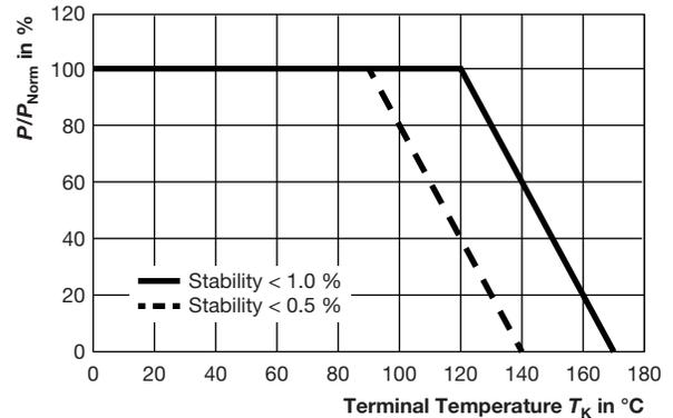
Fig. 2 - Terminal Temperature Derating
