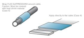
To suppress noise radiation (reflected noise) from Case5) the opening of shield, casing, etc
