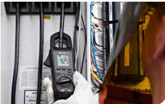
True RMS AC Current up to 600A
