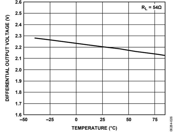
Figure 21. Driver Differential Output Voltage vs. Temperature
