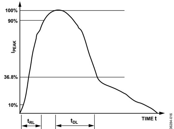
Figure 30. Human Body Model and Current Waveform
