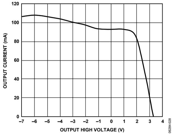
Figure 23. Output Current vs. Driver Output High Voltage
