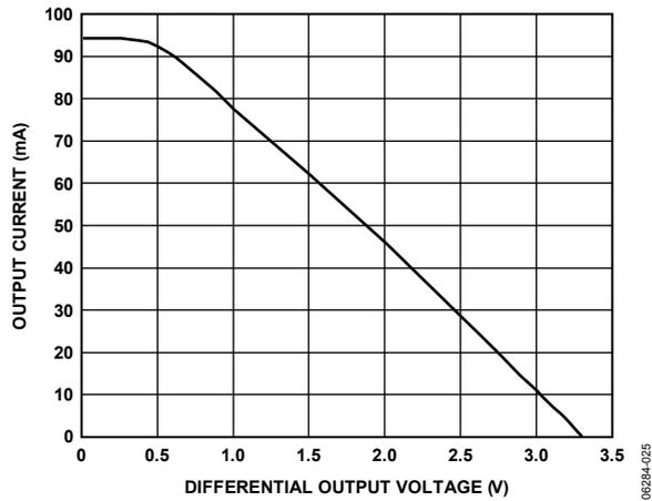
Figure 20. Driver Output Current vs. Differential Output Voltage
