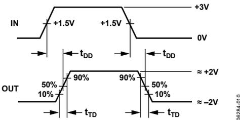
Figure 10. Driver Differential Output Delay and Transition Times
