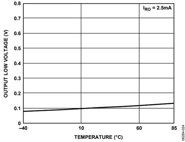
Figure 19. Receiver Output Low Voltage vs. Temperature
