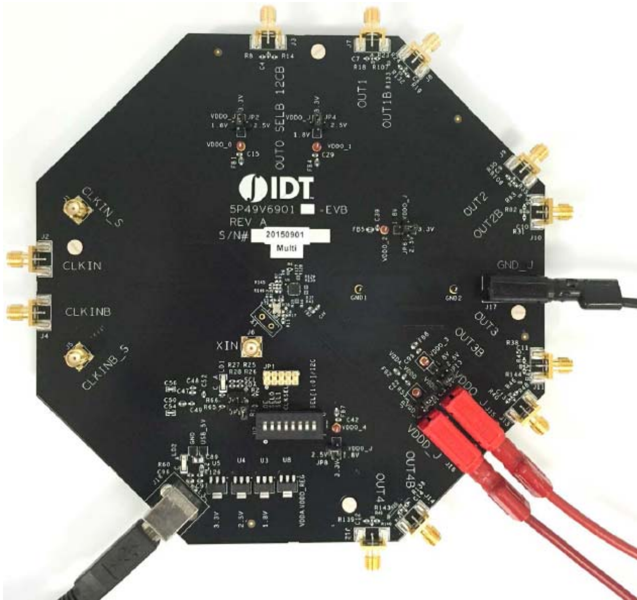
Figure 4. Connecting 5P49V6901 – EVB USB Port for Communications with Timing Commander Software and input voltage supplies
