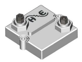
POWER RATING is based on 600 W at 85 °C heat sink temperature. Use of thermal conduction to heat sink is required. Flatness of cooling plate must be better than 0.05 mm overall, and the roughness should not exceed 6.4 um.
