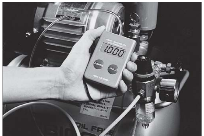
▲ Measurement of source pressure from a compressor.
