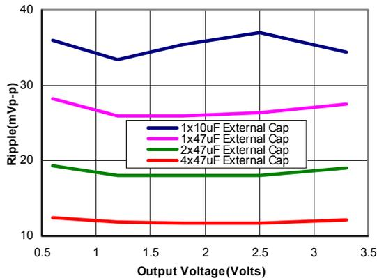
Figure 36. Output ripple voltage for various output voltages with external 1x10  $\mu\text{F}$ , 1x47  $\mu\text{F}$ , 2x47  $\mu\text{F}$  or 4x47  $\mu\text{F}$  ceramic capacitors at the output (20A load). Input voltage is 5V.
