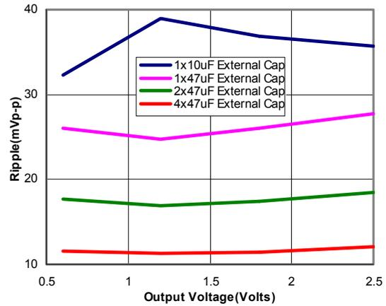
Figure 37. Output ripple voltage for various output voltages with external 1x10  $\mu\text{F}$ , 1x47  $\mu\text{F}$ , 2x47  $\mu\text{F}$  or 4x47  $\mu\text{F}$  ceramic capacitors at the output (20A load). Input voltage is 3.3V.
