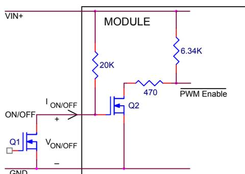
**Figure 38. Circuit configuration for using positive On/Off logic.**
