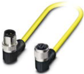
Sensor/Actuator cable, 3-position, yellow, Plug angled M12 SPEEDCON, A-coded, on Socket angled M12 SPEEDCON, A-coded, Cable length: 1.5 m
