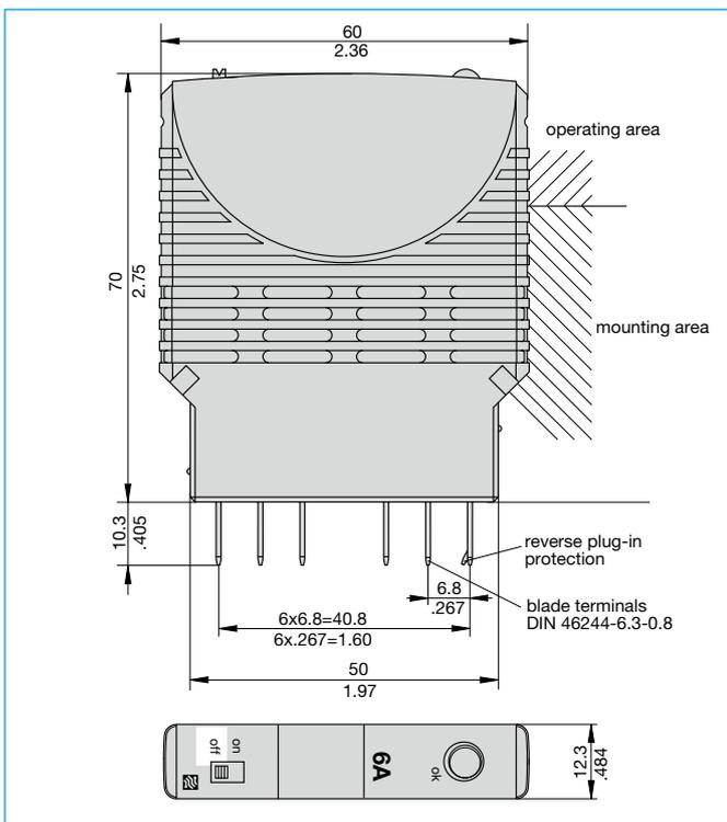
This is a metric design and millimeter dimensions take precedence ( $\frac{\text{mm}}{\text{inch}}$ )
