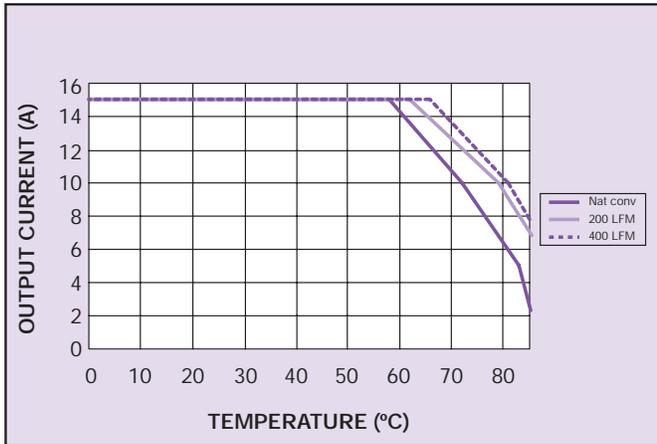
Figure 1 - Derating Curve
