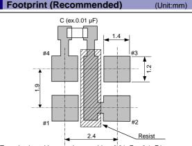
To maintain stable operation, provide a 0.01uF to 0.1uF by-pass capacitor at a location as near as possible to the power source terminal of the crystal product (between Vcc - GND).
