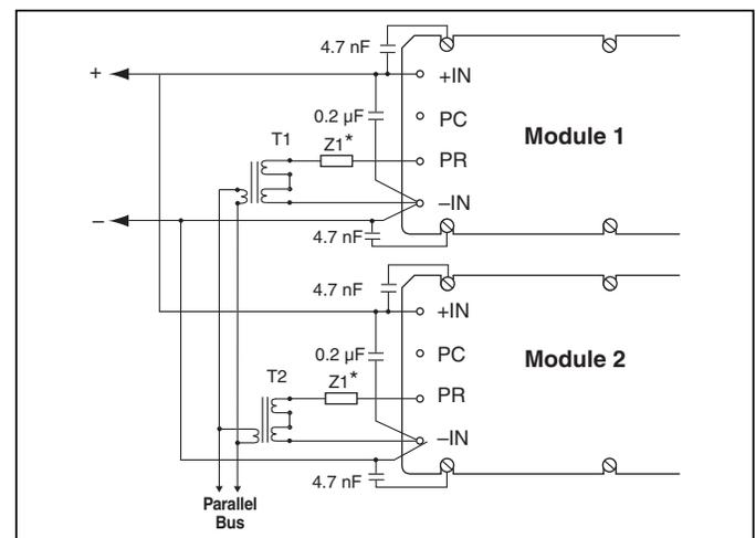
Figure 10 — Transformer-coupled interface.
