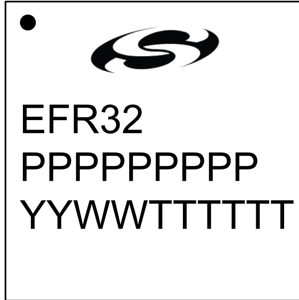
Figure 8.3. QFN32 Package Marking
