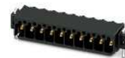
Header for THR applications, pin length 2.0 mm, gold-plated contact system, plug-in direction parallel to the PCB
