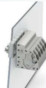
16 mm 2 molded feed-through terminal block, external part with push-in connection, internal part with cable lug connection
