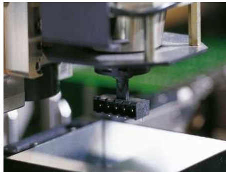
Camera recording for component measurement
