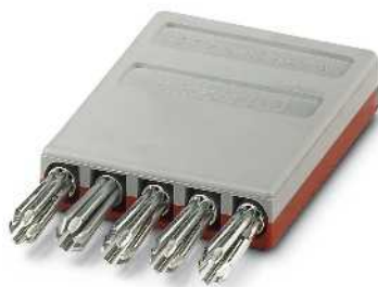
5-pos. test plug, 5/0/5.08 mm pitch, makes contact in the conductor connection space
