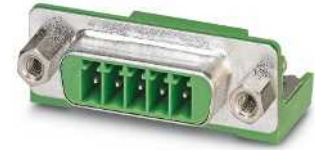
Shielded POWER SUBCON header for wall thicknesses of up to 4.5 mm, 4-40 UNC fastening thread, with leading medium PE contact
