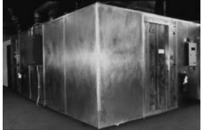
The Curtis screen room provides complete RFI isolation for equipment under test and the test instrumentation.
