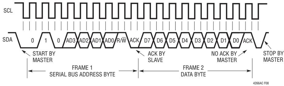
Figure 8. Reading the Interrupt Register (Short Form)
