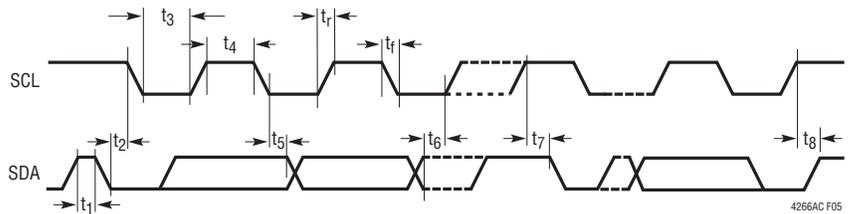
Figure 5. I<sup>2</sup>C Interface Timing
