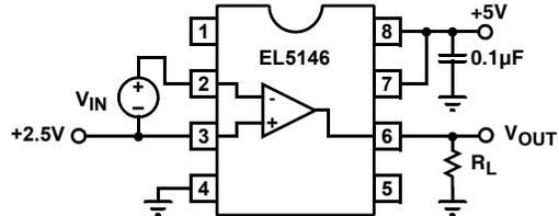
FIGURE 50. EL5146 AMPLIFIER IMPLEMENTED AS A COMPARATOR
