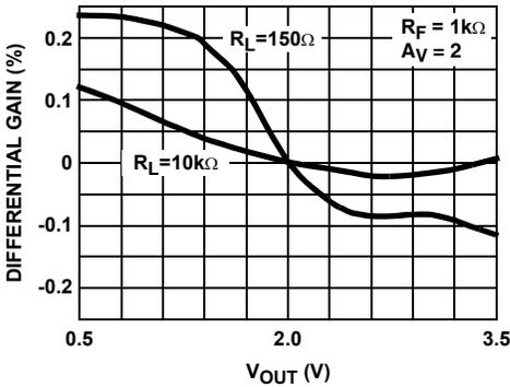
FIGURE 29. DIFFERENTIAL GAIN FOR  $R_L$  TIED TO 0V
