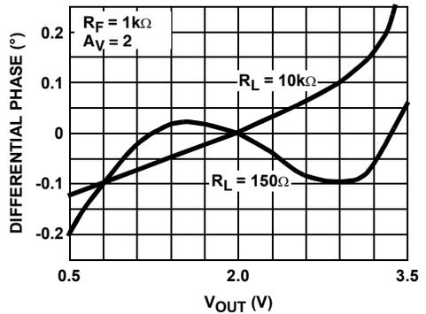
FIGURE 32. DIFFERENTIAL PHASE FOR  $R_L$  TIED TO 2.5V
