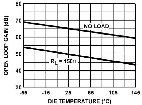
FIGURE 12. OPEN LOOP VOLTAGE GAIN vs DIE TEMPERATURE
