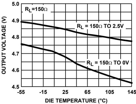
FIGURE 41. POSITIVE OUTPUT VOLTAGE SWING vs DIE TEMPERATURE
