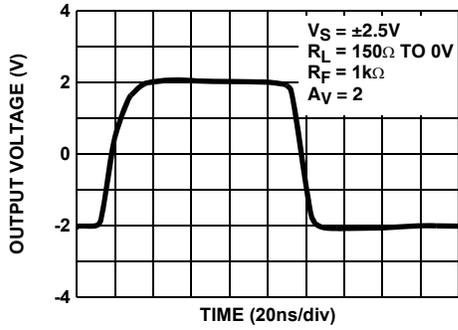
FIGURE 21. LARGE SIGNAL PULSE RESPONSE (SPLIT SUPPLIES)
