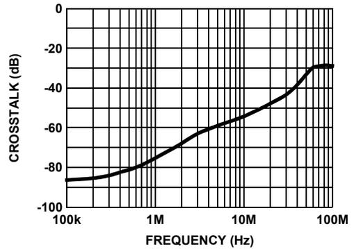
FIGURE 36. CHANNEL-TO-CHANNEL CROSSTALK - DUALS AND QUADS (WORST CHANNEL)
