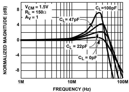
FIGURE 8. FREQUENCY RESPONSE FOR VARIOUS  $C_L$
