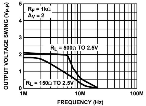
FIGURE 18. OUTPUT VOLTAGE SWING vs FREQUENCY FOR THD < 0.1%
