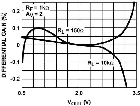
FIGURE 31. DIFFERENTIAL GAIN FOR  $R_L$  TIED TO 2.5V
