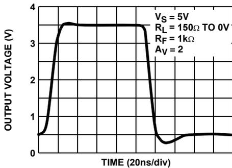
FIGURE 19. LARGE SIGNAL PULSE RESPONSE (SINGLE SUPPLY)
