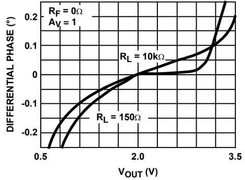
FIGURE 28. DIFFERENTIAL PHASE FOR  $R_L$  TIED TO 2.5V
