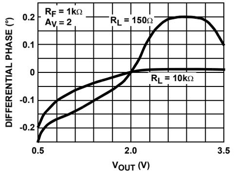
FIGURE 30. DIFFERENTIAL PHASE FOR  $R_L$  TIED TO 0V
