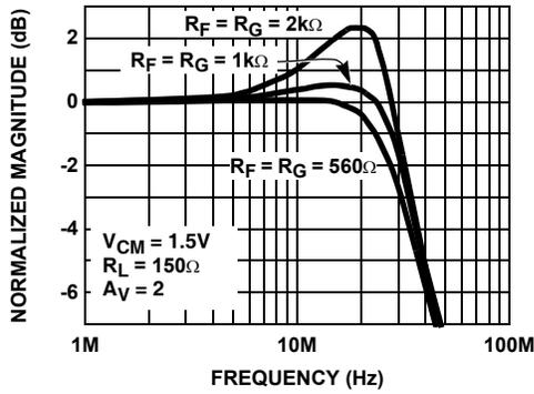
FIGURE 9. FREQUENCY RESPONSE FOR VARIOUS  $R_F$  AND  $R_G$
