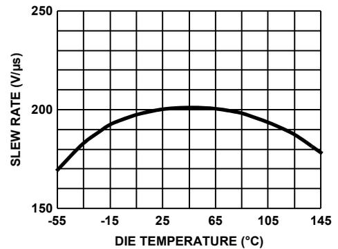
FIGURE 24. SLEW RATE vs DIE TEMPERATURE
