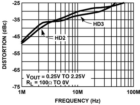
FIGURE 33. 2nd AND 3rd HARMONIC DISTORTION vs FREQUENCY
