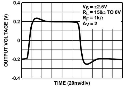
FIGURE 22. SMALL SIGNAL PULSE RESPONSE (SPLIT SUPPLY)
