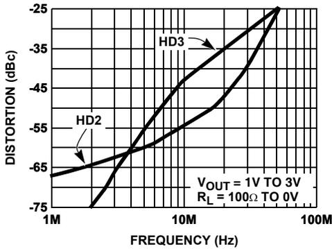
FIGURE 35. 2nd AND 3rd HARMONIC DISTORTION vs FREQUENCY
