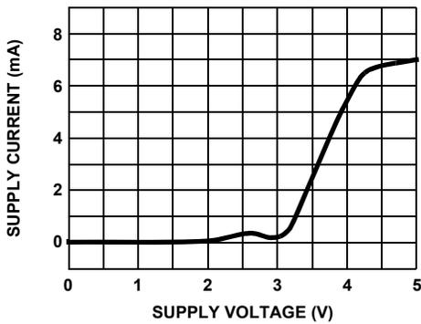
FIGURE 37. SUPPLY CURRENT (PER AMP) vs SUPPLY VOLTAGE
