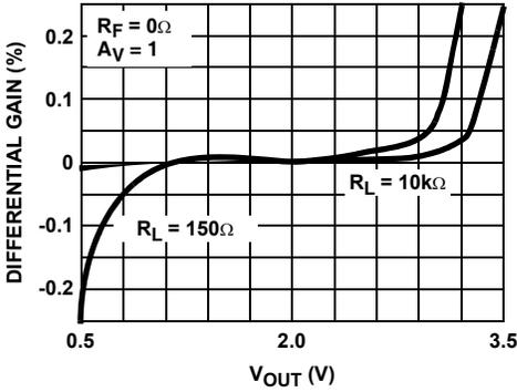
FIGURE 27. DIFFERENTIAL GAIN FOR  $R_L$  TIED TO 2.5V
