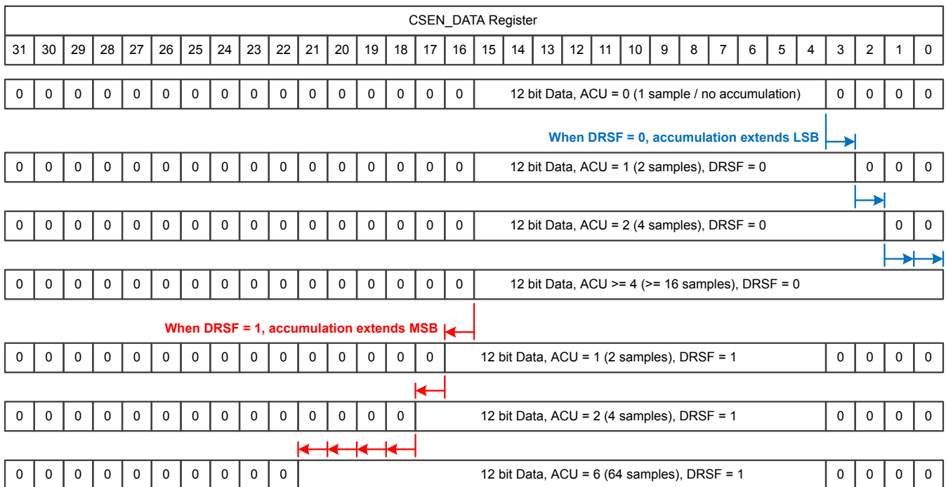
Figure 35.7. Data Encoding for Different Accumulator Settings
